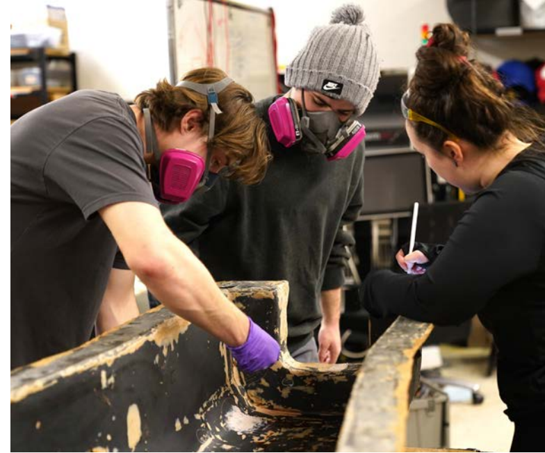
UWFM members do almost all manufacturing and assembly in-house. Here, ME and MSE students prep the monocoque mold of this year's car before carbon fiber layup. Photo courtesy of UWFM
