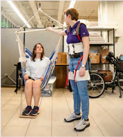
A team designed a harness-based support system attached to an overhead frame structure. Photo by Jorge Azpeitia/University of Washington
