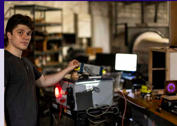
Ben Price adjusts the current on the power supply box to apply voltage across a plasma actuator, shown on the right.
