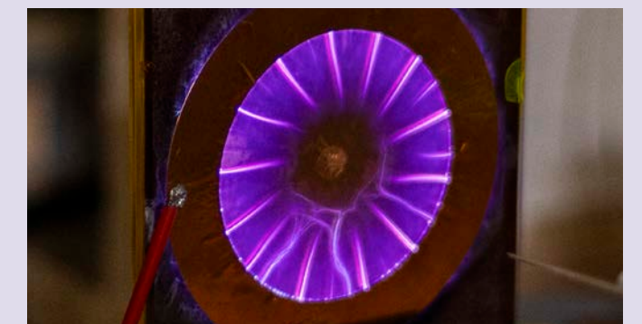
The purple streaks of light indicate a high energy discharge where electrons flow through. Typically the researchers try to apply as much voltage as they can without getting them.
